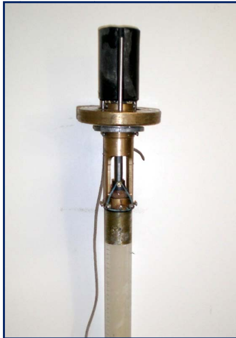
Figure 1. Gravity corer used to collect sediment core samples.
